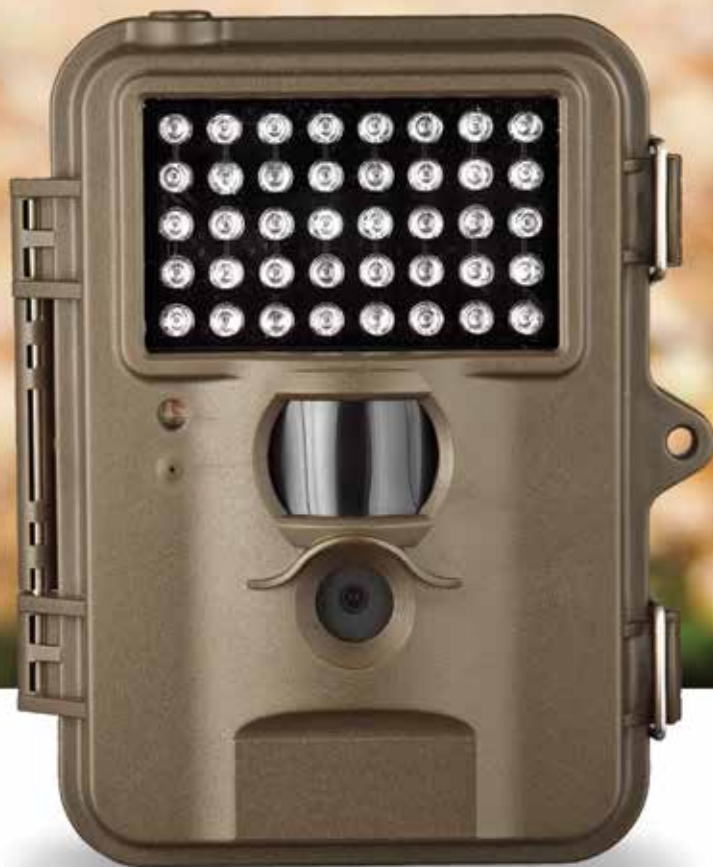
8MP Trail Camera w/2" Color Screen and 40 Infrared LED Lights BG11751
